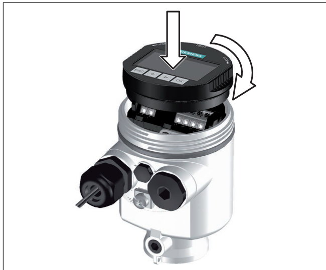
Fig. 22: Insertion of the display and adjustment module with single chamber housing into the electronics compartment
